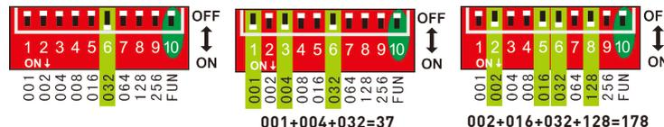
\* When Dip switch 1-9 are OFF, the defaulted initial DMX address is 1.
