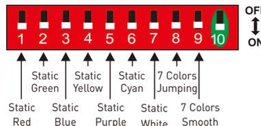
For changing effects [Dip Switch 8/9=ON]: Dip switch 1-7 is used to realize 7 speed levels. (7=ON, the fastest level)
